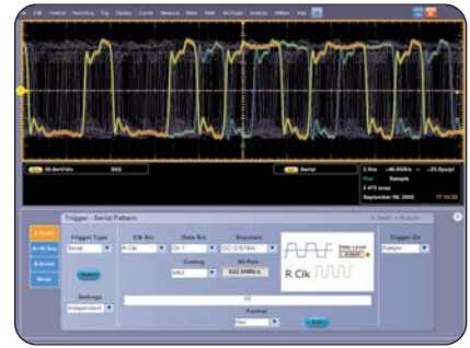
► Serial pattern triggering to debug pattern dependent issues.
