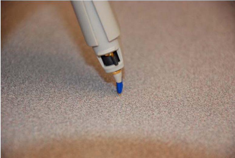
Figure 6 The proper vertical orientation of the blue tips on the differential browser probe head
