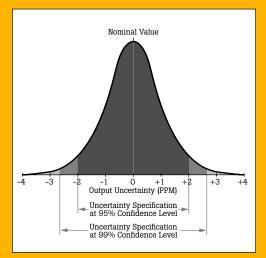
A critical factor in specified calibrator performance is the difference between the actual output value and the nominal output value. The confidence interval is a statistical expression of the likelihood that any output of any instrument will deviate beyond this specified difference or uncertainty.
