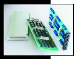
The Model 7011 40-channel multiplexer has four independent banks of 1×10 switching. Each channel is 2-pole. These four banks can be combined for a wide variety of switching configurations—for example, dual 1×20, or 1×10 and 1×30, or one large 1×40. The 7001 mainframe can automatically configure the 7011 to switch 4-pole signals by combining channel pairs. This gives you a dual 1×10 4-pole multiplexer or a single 1×20 4-pole multiplexer.
