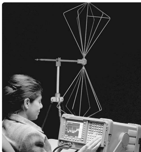
A number of antennas are available with the 84115EM system to test for RF emissions. The E7400 EMC analyzer will also work with other third party antennas.
