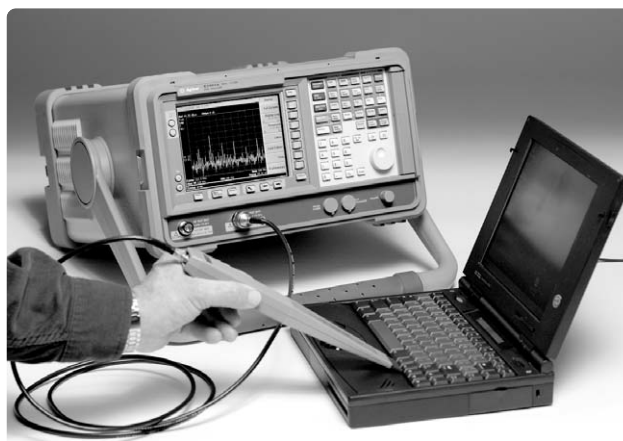
A number of antennas are available with the 84115EM system to test for RF emissions. The E7400 EMC analyzer will also work with other third party antennas.
