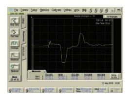
Accurate time domain reflectometry/transmission and S-Parameter measurements
