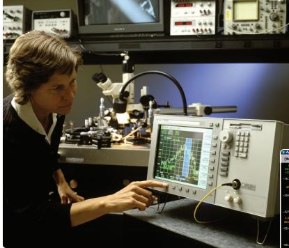
Any of the four independent markers can be arbitrarily set on any of the six available traces, so any absolute or relative value can be measured. Furthermore, each marker can measure bandwidth and calibrated optical signal-to-noise ratio quickly. The noise markers provide calibrated noise power normalized to a standard 0.1 nm noise equivalent bandwidth automatically for any resolution bandwidth setting. Thus, eliminating steps and reducing your time to market.
