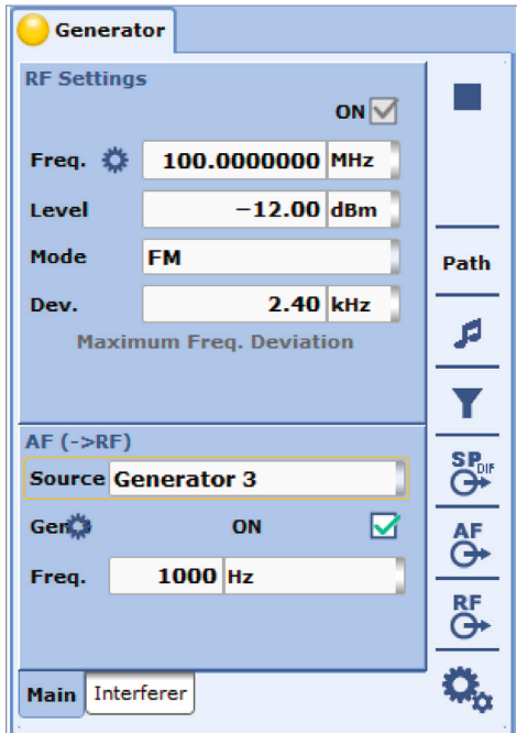
Frequency modulation with an internal audio source.
