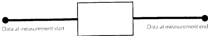
The measured waveform is "replayed" across the screen in scrolling mode after the acquisition ends. The scrolling direction and speed can be set by the user.
