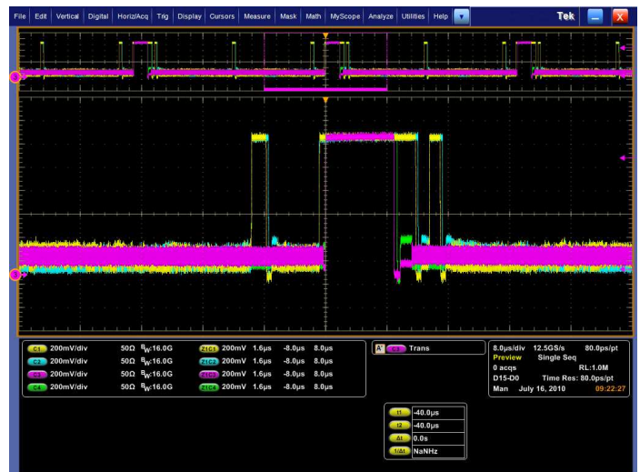
MIPI® D-PHY Characterization and Analysis Solution (Option D-PHY) – Verify to the D-PHY specification by rapidly characterizing and discovering sources of jitter and signal integrity concerns using the fully flexible and customizable test setup. Using DPOJET, Option D-PHY enables transmitter high-speed data-clock timing measurements, along with a full range of electrical characteristics in high-speed or low-power modes.
