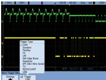
Trigger on and decode CAN serial packets.
