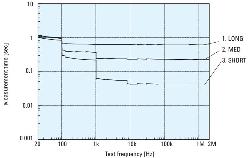
**Figure 10. Measurement time (DC bias: OFF, Option 005)**
