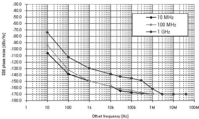
**Figure1-2. SSB phase noise sensitivity (E5052A-011, typical)**
