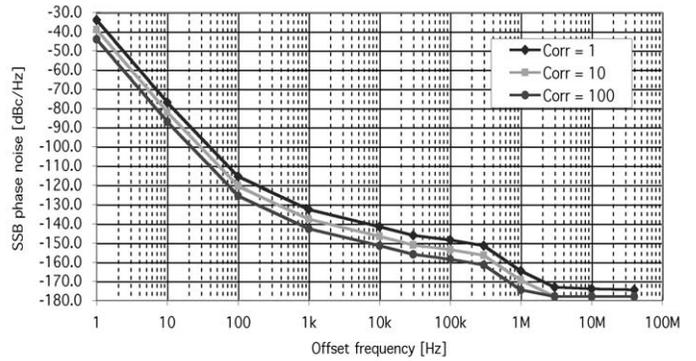
**Figure1-3. SSB phase noise sensitivity improved with the cross-correlation function (typical)**
