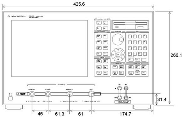
Figure 1-5. Dimensions (front view, in millimeters, nominal)
