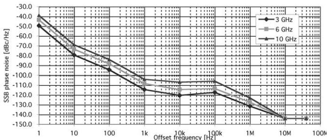
Figure 2-3. E5052A downconverter LO phase noise (typical)
