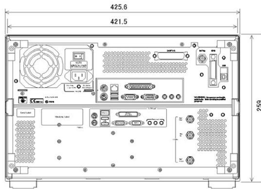
Figure 1-6. Dimensions (rear view, in millimeters, nominal)
