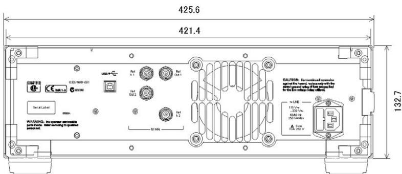
Figure 2-5. Dimensions (rear view, in millimeters, nominal)
