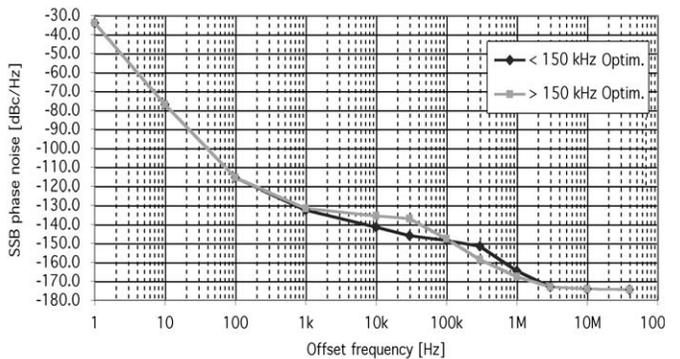
**Figure1-4. SSB phase noise sensitivity of different LO optimization**
