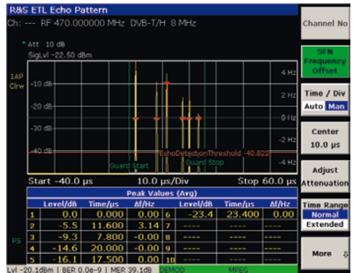
Channel impulse response with SFN frequency offset-measurement (red lines).
