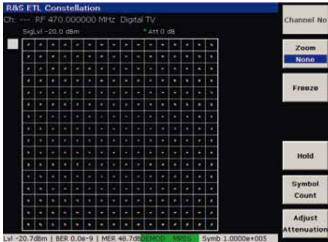
Constellation diagram of a DVB-C signal.
