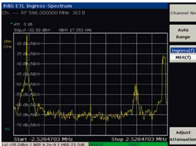
Ingress (f), frequency spectrum of an interfering signal that is superimposed on the useful signal.
