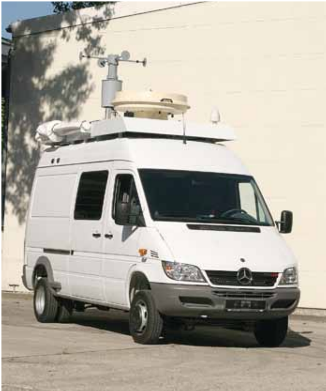
Mobile coverage measurements in the field.
