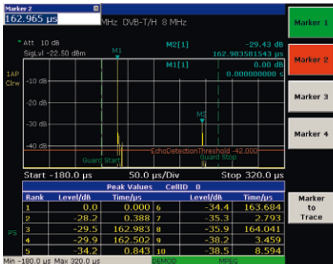
DVB-T, DVB-H channel impulse response with markers.
