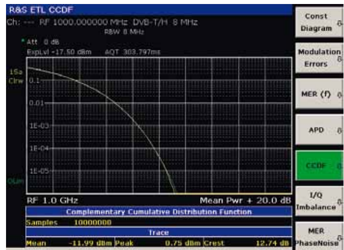
Complementary cumulative distribution function (CCDF) measurement.
