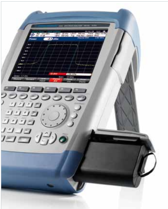
Easy-to-replace Li-ion battery for up to 4.5 h of operation.
