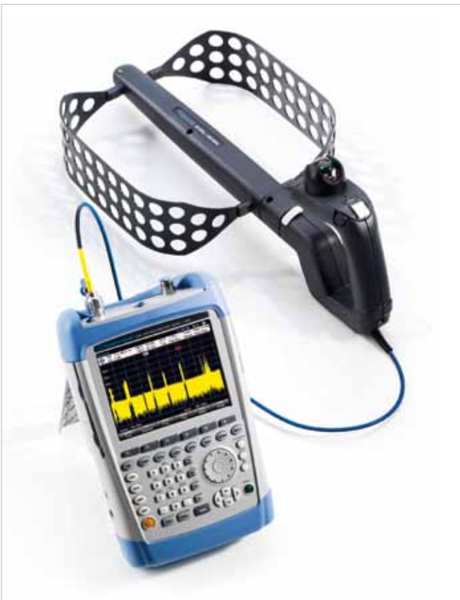
The R&S®FSH8 with the R&S®HE300 antenna.
