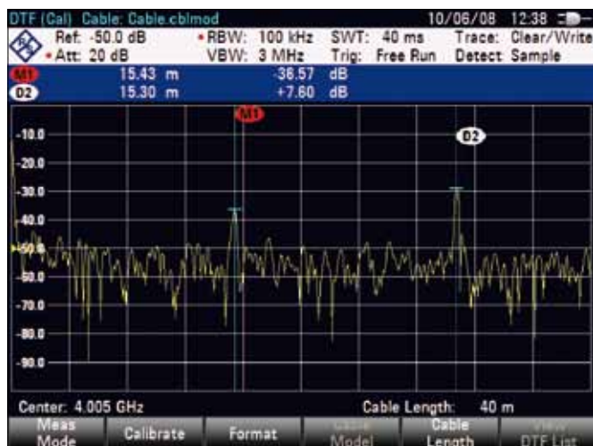
Distance-to-fault (DTF) measurement.
