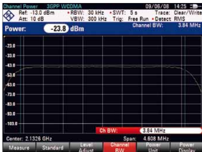
Channel power measurement.
