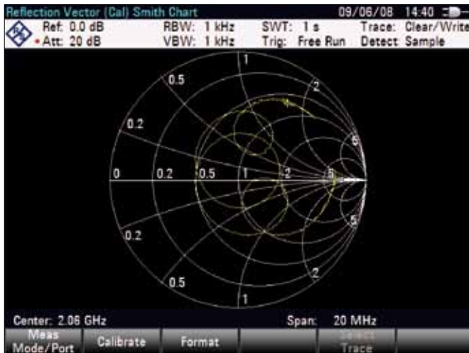
Vector network analysis: measurement with Smith chart.
