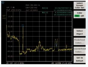
AF spectrum of an FM stereo signal: The 19 kHz pilot carrier, the stereo signal on the 38 kHz subcarrier and the RDS subcarrier at 57 kHz are clearly distinguishable. The pilot deviation is selected using the marker.
