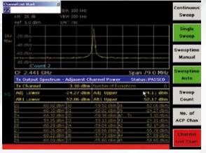
Adjacent channel power (ACP): This measurement determines the power of all adjacent channels. The power of up to 79 channels in total can be measured. For EDR inband spurious the measurement can be gated.
