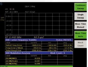
Carrier frequency stability and modulation accuracy: This measurement determines the frequency accuracy within the packet header, the frequency drift within the DPSK part, as well as the DEVM metrics.
