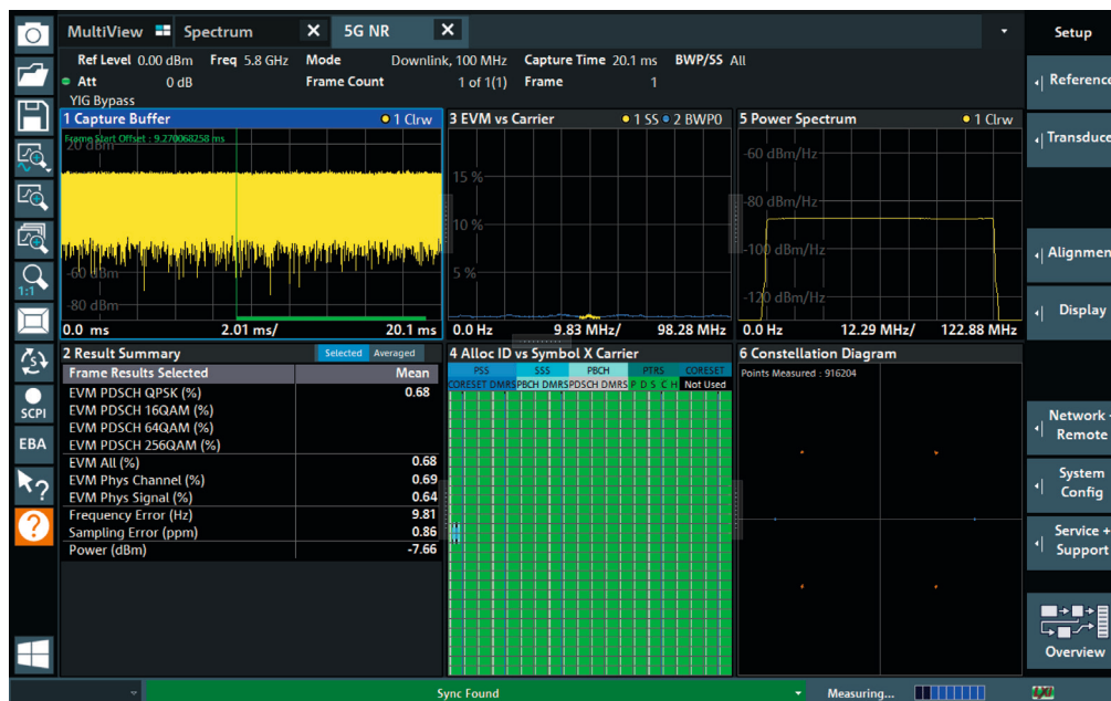
Analysis of a 5G NR signal with the R&S®FSV3-K144 (downlink) and R&S®FSV3-K145 (uplink) options
