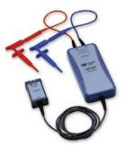
The ZS Series probes provide high impedance and an extensive set of probe tips and ground accessories to handle a wide range of probing scenarios. The high 1 M $\Omega$  input resistance and low 0.9 pF input capacitance mean this probe is ideal for all frequencies. The ZS Series probes provide full system bandwidth for all Teledyne LeCroy oscilloscopes having bandwidths of 1 GHz and lower.
