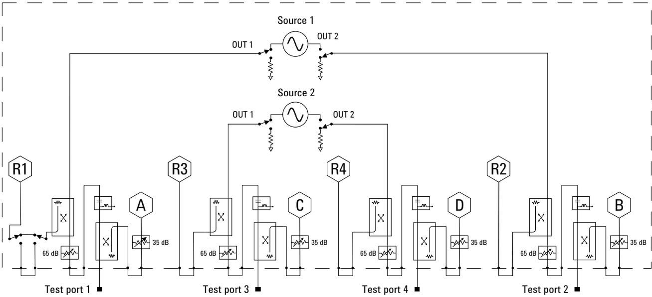
**Add an internal combiner and mechanical switches to 4-port analyzer (Option 423 requires Options 400, 419 and 080)**
