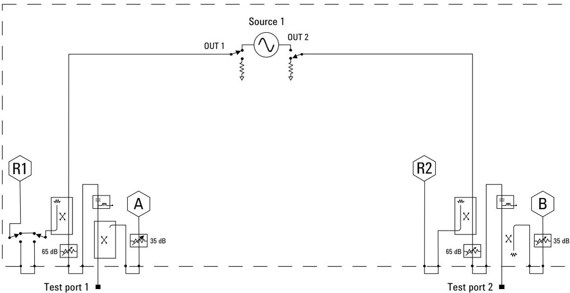
**Add an internal second source, a combiner, and mechanical switches to 2-port analyzer
