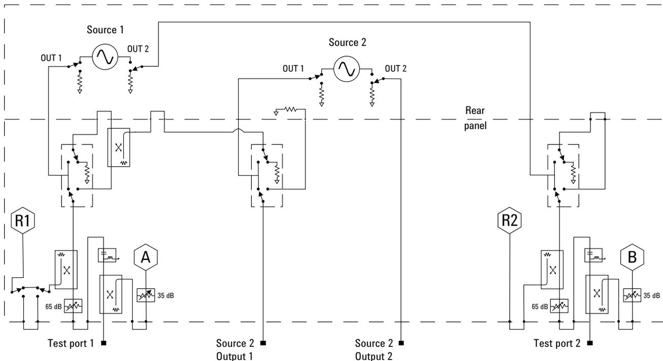
**4-port standard test set, power range, and an internal second source (Option 400, recommends Option 080)**
