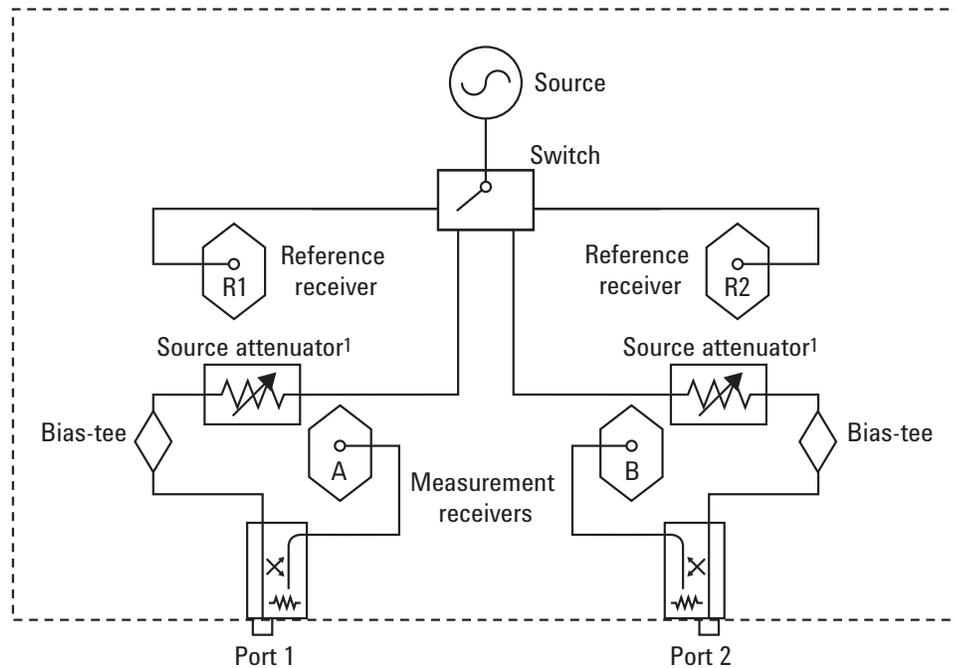
1. Source attenuator for E8362/3/4C is 60 dB in 10 dB steps.
