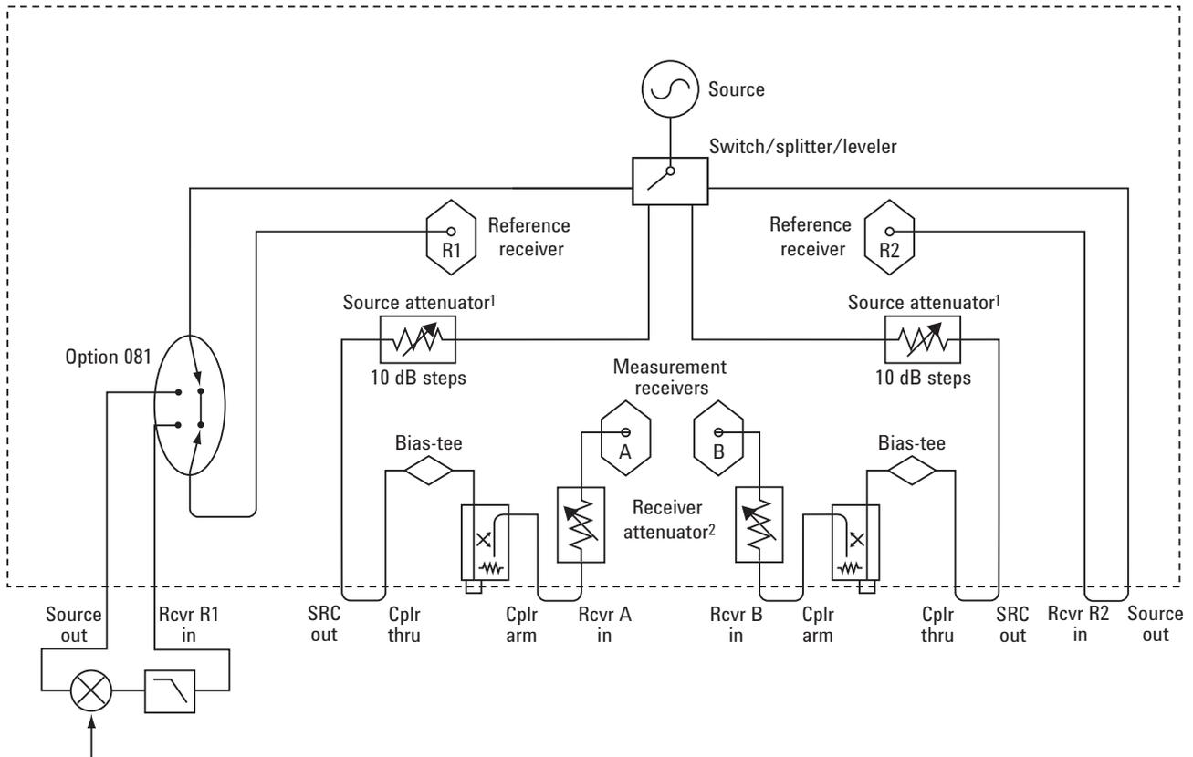
1. Source attenuator for E8362/3/4C is 60 dB in 10 dB steps. Source attenuator for E8361C is 50 dB in 10 dB steps.
