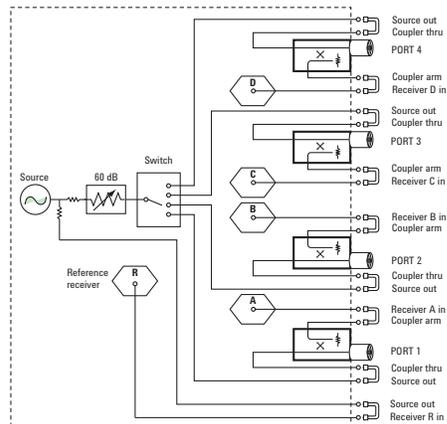
4-port configurable test set, extended power range and internal second source
