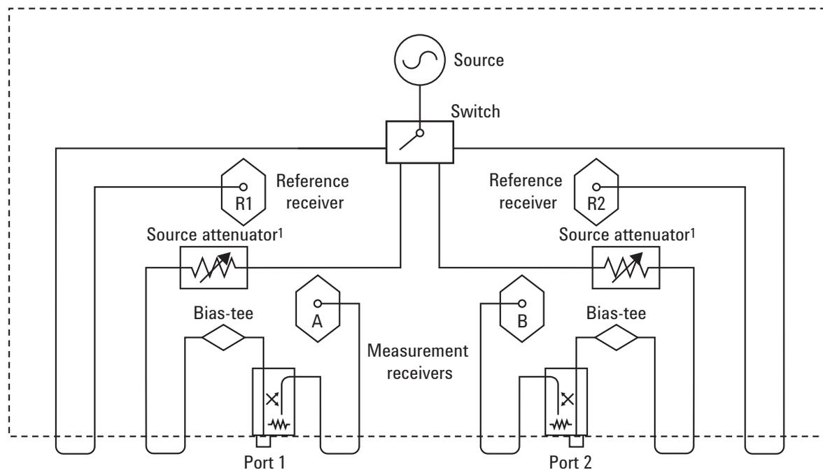
1. Source attenuator for E8362/3/4C is 60 dB in 10 dB steps.
