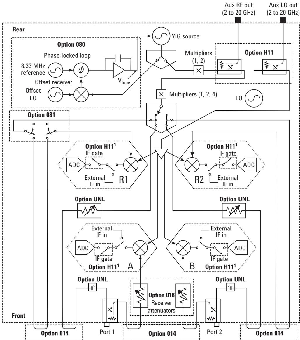
1. Option H11: IF-gate controls and external-IF inputs are accessed on rear panel. IF gates are enabled with Option H08. External-IF input frequency is 8.33 MHz.
