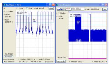
Advanced Triggers and Swept DPX combines the revolutionary DPX Density™ Trigger with the ability to trigger on runt pulses and apply time qualification to any trigger. The runt trigger seen here can be used to track down nonconforming pulses in a pulse train, greatly reducing time to insight. Time qualification can be used to separate ranging pulses from higher resolution pulses in a radar signal, or trigger only on signals that remain on longer than a specified time.
