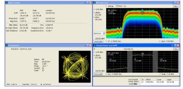
Time-correlated, multidomain views provide a new level of insight into design or operational problems not possible with conventional analysis solutions. Here, ACLR and Vector Modulation Quality (Opt. 21) are performed on a single acquisition, combined with the continuous monitoring of the DPX<sup>®</sup> spectrum display.
