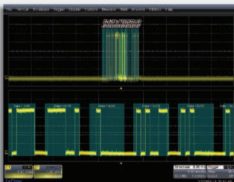
The serial data trigger will quickly isolate events on a bus eliminating the need to set manual triggers and hoping to catch the right information. Trigger conditions can be entered in binary or hexadecimal formats and conditional trigger capabilities even allow triggering on a range of different events.
