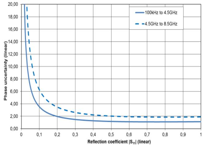
Typical accuracy of reflection magnitude and reflection phase measurements for the R&S®ZND
