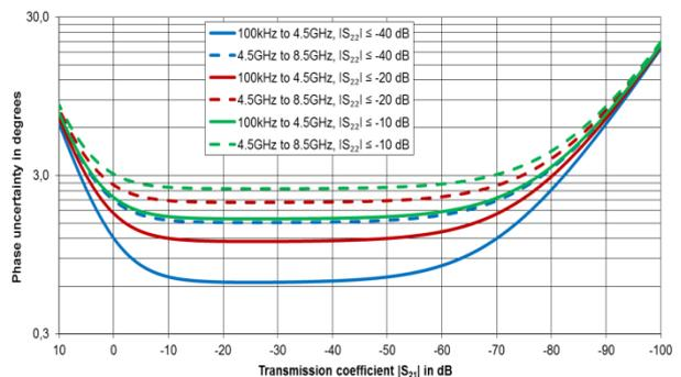
Typical accuracy of transmission magnitude and transmission phase measurements for the R&S®ZND
