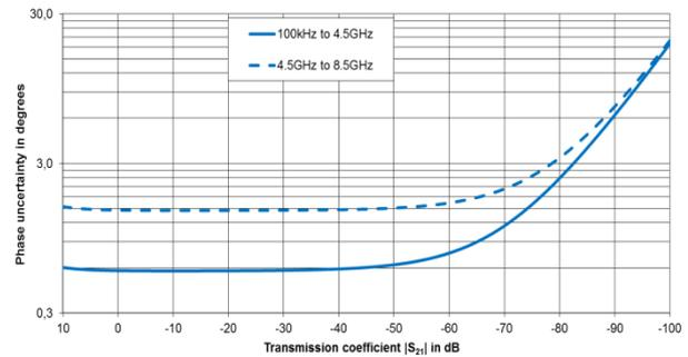
Typical accuracy of transmission magnitude and transmission phase measurements for the R&S®ZND
